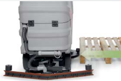
Automatic swing-in of the brush head when accidentally impacted (Innova 65/75/85 B)
