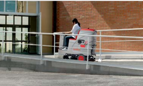
Low center of gravity for optimum stability. Capable of ramp gradients up to 18%
