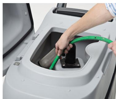
11. Wash with clean water the recovery tank and the vacuum grid
