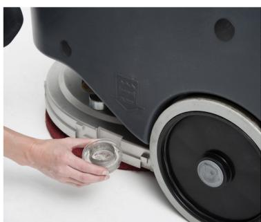
15. Clean the filter by: Remove the transparent cover and the gasket
