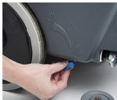
7. Press the eco solution flow control valve
