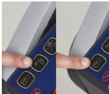
9. To change the solution flow level push the solution button and change flow level according to the cleaning performance and application.
