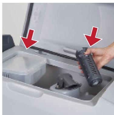
2 Open the recovery tank and check the debris tray and float are clean and working.
