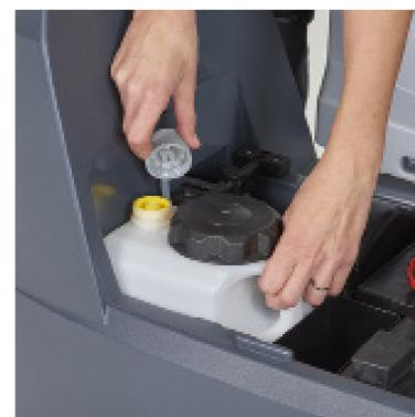
4 Check the EcoFlex™ system is cleaned, eventually purge the system.
