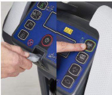
6. Insert the operator key, then start the machine by pressing the One-Touch button. To engage the brush, slightly press the drive paddle and then release it.
