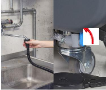
2. Fill the tank with a clean water. The clean water temperature must not exceed 40 °C. Make sure the solution valve under the machine is open.
