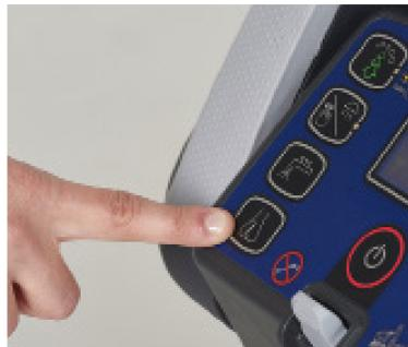
12. Machine with Ecoflex, always end the daily work with turning off the detergent 2 minutes before finishing by pressing the detergent button. To rinse out detergent from the system and brush before handling and cleaning.
