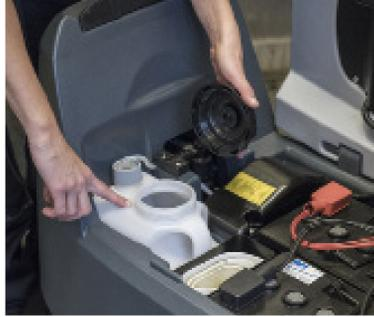
3. Fill the EcoFlex™ tank with a detergent suitable for cleaning machines (highly concentrated and low foaming detergent).
