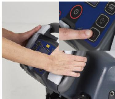
8. Push forward the drive paddle to start cleaning. Adjust maximum speed by the speed regulation buttons.
