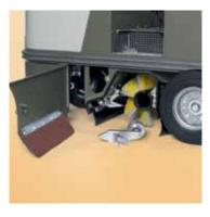
The pressure and height adjustment of the central brush are controlled simply by the knob near the brush. Brush height adjustment depending on wear can, therefore, be done very easily. This ensures a longer brush life cycle
