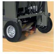
The central brush is the floating type and self-adjusts to keep in contact with the ground all the time
