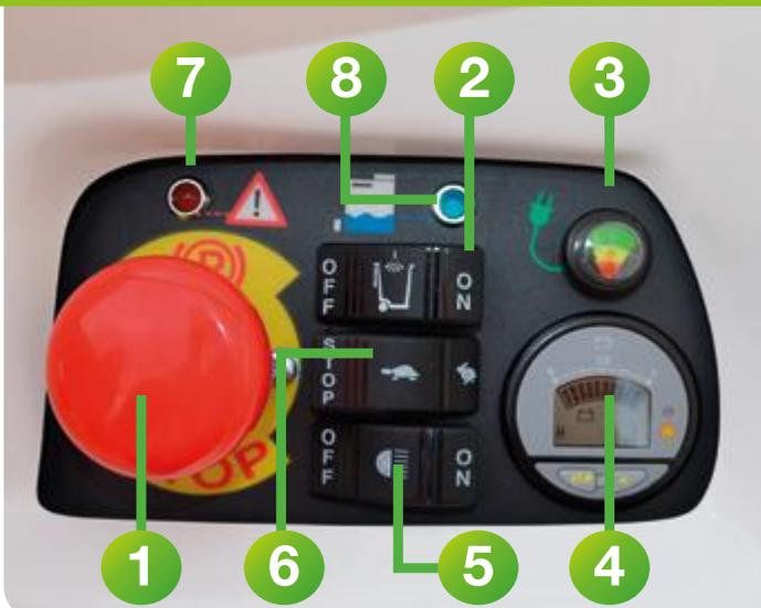
The emergency stop button is clearly visible on the control panel and it is easy to operate by hand.
