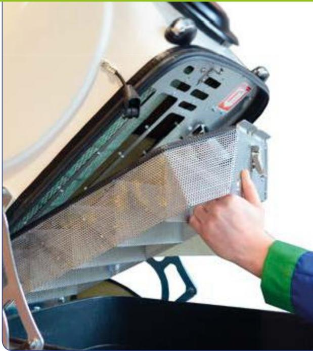
The suction system has an anti-clogging grid to prevent blockages caused by plastic bags, dead leaves, etc.
