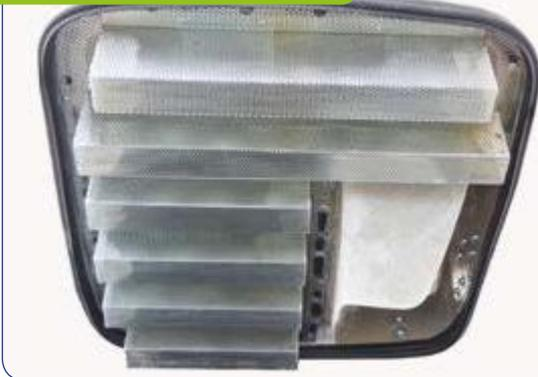
The suction system has an anti-clogging grid to prevent blockages caused by plastic bags, dead leaves, etc.
